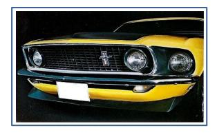
The front spoiler is to meet the specifications and dimensions of the original Ford part number C9ZZ-63001A74-A. The spoiler will be of high impact flexible plastic with the outside of the longest part on the corners 58-1/2" in length. The total width in the centre including the bottom lip 5". The total length at the centre before it turns corners (front part before turn) 50".
