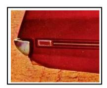
Repeater lights on lower front guards and rear quarter panels must be installed.
