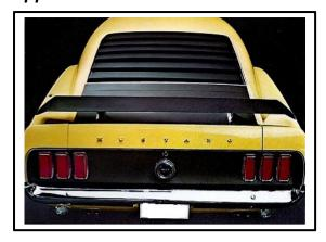
The rear spoiler is to meet the specifications and dimensions of the original Ford part number C9ZZ-6344210-K.
