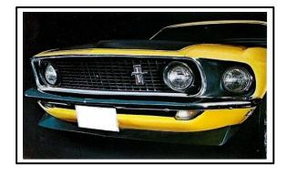
The front spoiler is to meet the specifications and dimensions of the original Ford part number C9ZZ-63001A74-A. The spoiler will be of high impact flexible plastic with the outside of the longest part on the corners 58-1/2" in length. The total width in the centre including the bottom lip 5". The total length at the centre before it turns corners (front part before turn) 50".
