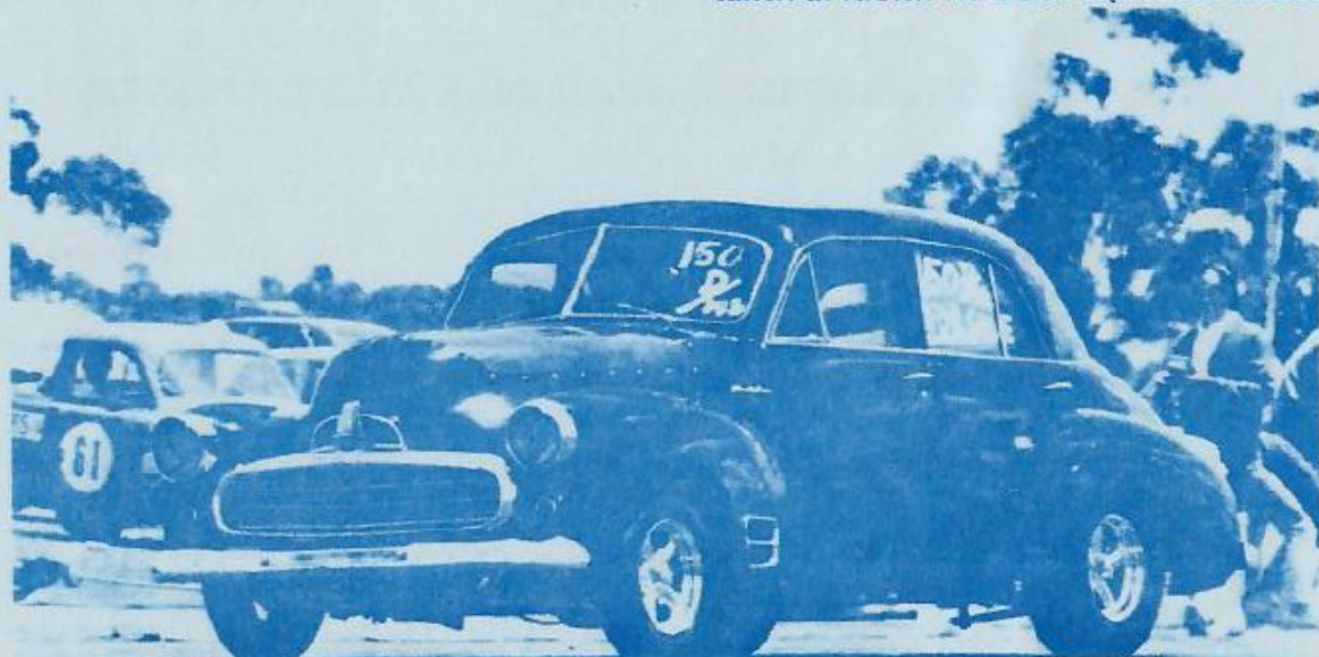
'Black Shadow' built originally by Alby Oliver in the late 60's. This car collected a huge supply of custom trophies across Australian shows. It used a simple grille treatment, flawless black paint and perspex bonnet inserts. In later life the grey motor was replaced with a 186 and regular drag racing competition undertaken. (Ecurie Photo)
